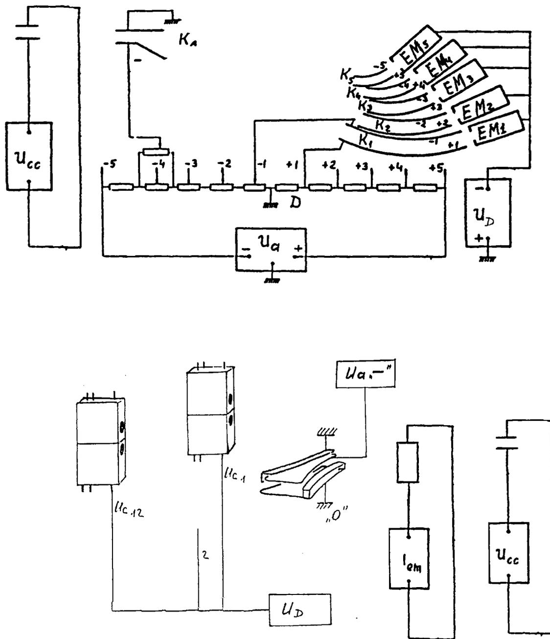
**Figure 6.** Scheme of the power supply of both analysers, 5-channel analyser (up) and Acord12 (down).  $U_{cc}$  is the voltage to the clanging condenser;  $U_a$  is the voltage to the analyser condenser (in 5-channel analyser also to the condensers of the channels), in the 5 channel analysers the  $U_a$  is supplied by two power supply;  $U_D$  is the voltage applied to the detectors; and  $I_{em}$  is the current source applied to the electromagnet.
