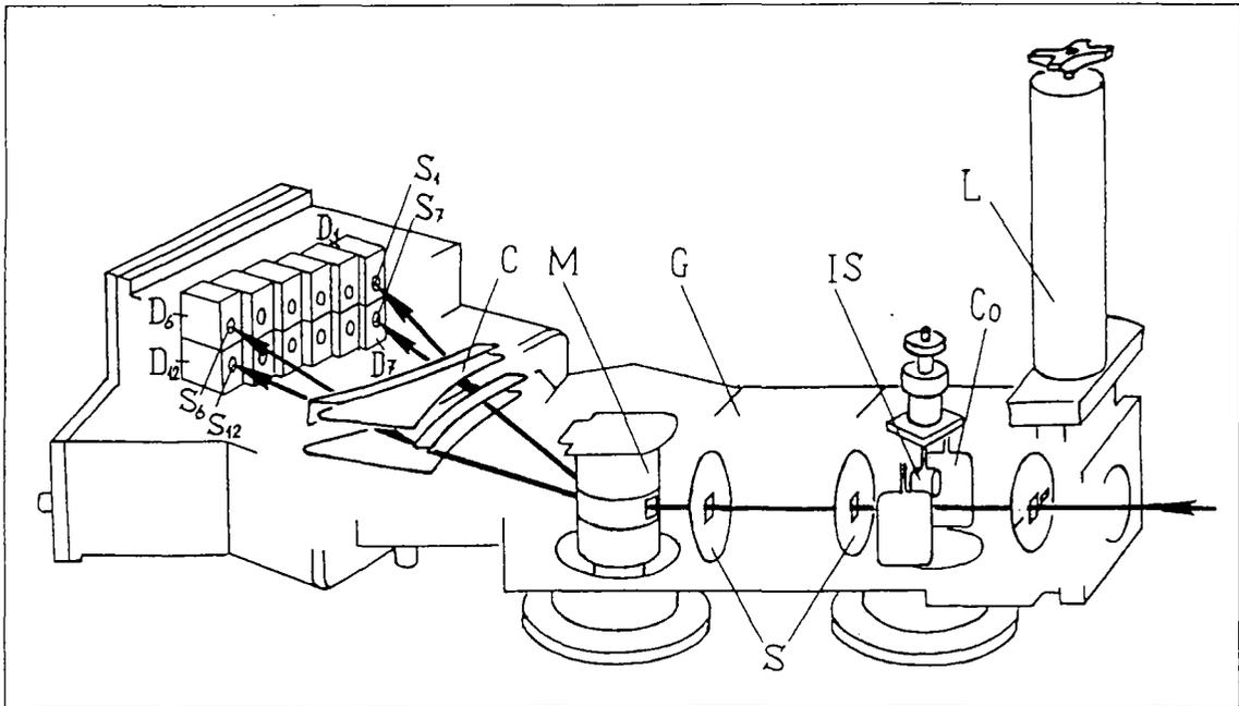
**Figure 1.** Scheme of the Acord12. L is the vacuum valve; IS is the alkali ion source;  $C_0$  is the cleaning condenser; G is the stripping chamber; S are the stripping chamber slits; M is electromagnet; C is analysing condenser;  $S_1$ - $S_{12}$  are input channel slits;  $D_1$ - $D_{12}$  are detectors.
