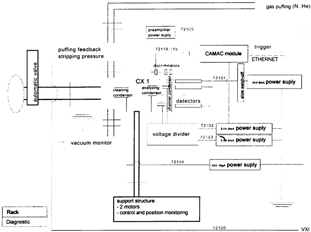
Figure 5a. Scheme of the electric connections for the 5- channel analyser.
