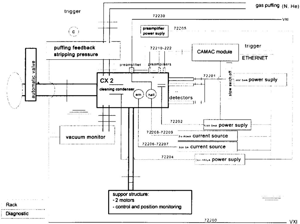
Figure 5b. Scheme of the electric connections for the Acord12.
