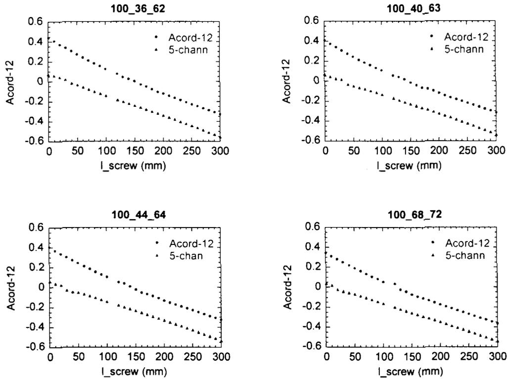
**Figure 3** Effective radius scanned as a function of the length of the screw (parameter in the remote control screen), for the two neutral particle analyser for different magnetic configurations of TJ-II. The three numbers in the name (i.e. 100\_44\_64) refer to the different currents in the TJ-II coils that determine the configuration.
