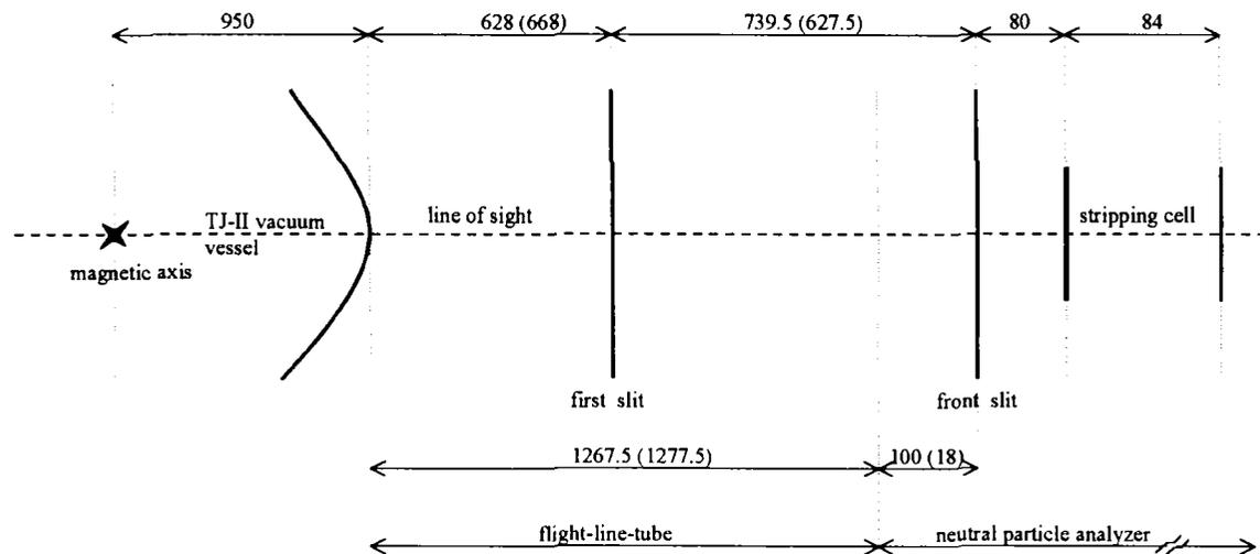
**Figure 4.** Scheme of the slits in the analysers and the different slits in the path of the neutrals, from left (vacuum vessel) to right (exit of the stripping cell). The numbers are the distance in millimeters in the Acord12, in brackets those corresponding to the 5 channel analyzer when different of Acord12.
