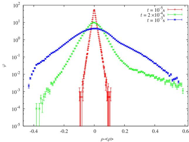
FIG. 4. (Color online) PDF of the radial displacements for the ECH plasma at three different times. The starting position is  $\rho=0.4$ .
