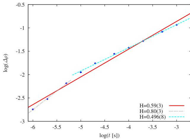
FIG. 8. (Color online) Log-log plot of the second moment of the PDF vs the time for the ECH plasma at  $\rho=0.4$ . The Hurst exponent is extracted for two different time scales.
