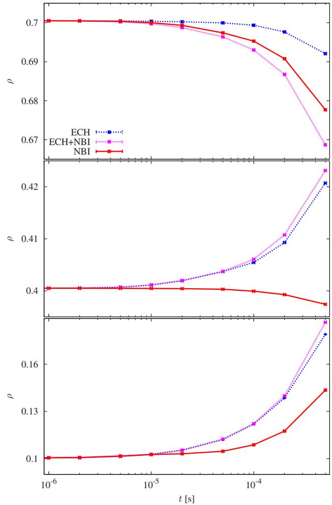
FIG. 3. (Color online) Average radial coordinate  $\rho$  of the ions as a function of time, with the experimental electric field included in the calculations.
