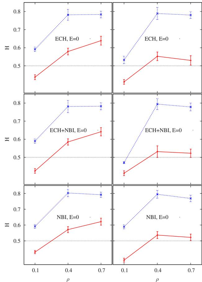
FIG. 9. (Color online) Radial profile of the Hurst exponent for all the plasmas simulated with (continuous) data up to  $t=10^{-5}$  s and (dashed) up to  $t=2 \times 10^{-3}$  s.
