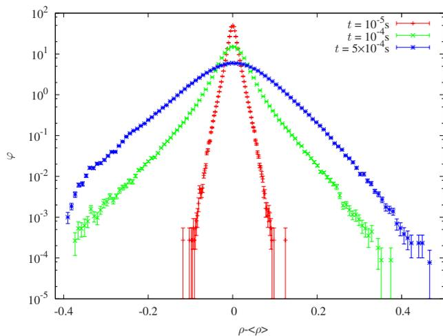
FIG. 6. (Color online) PDF of the radial displacements for the NBI plasma at three different times. The starting position is  $\rho=0.4$ .
