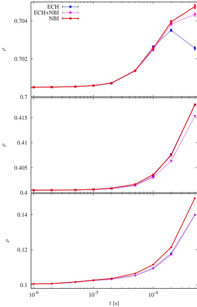
FIG. 2. (Color online) Average radial coordinate  $\rho$  of the ions as a function of time without electric field for the three regimes described in Sec. III and for the three starting radial positions.
