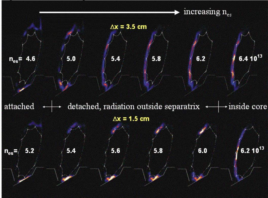
Fig.4: Evolution of carbon radiation zone through detachment for two different  $\Delta x$  cases. Top: larger  $\Delta x$ , radiation zone moves gradually to X-points on the inboard side with increasing  $n_{es}$ . Bottom: smaller  $\Delta x$ , radiation zone stays poloidally in divertor region while it moves inwards.
