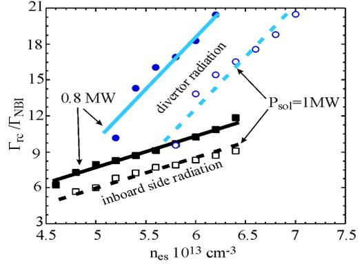
Fig. 6: Neutral gas penetration flux into the core as a function of  $n_{es}$ ,  $P_{sol}$  and configuration calculated by the 3D code.
