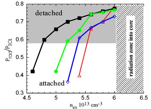
Fig. 3: Carbon radiation normalized to  $P_{sol}$  as a function of  $n_{es}$  and configuration.
