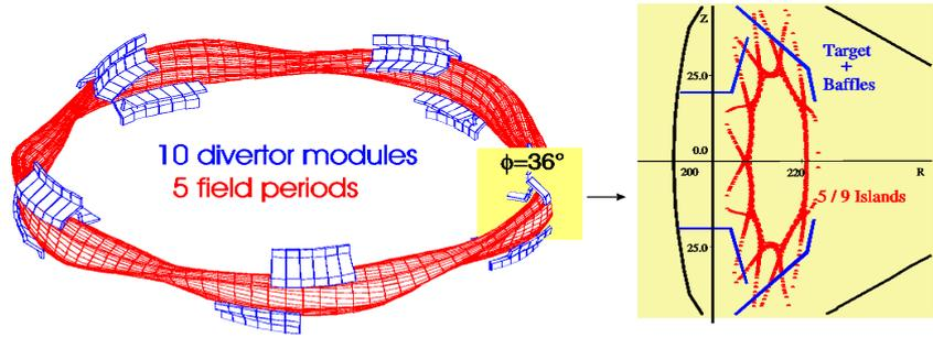
*Fig.1: Island divertor geometry in W7-AS. Ten up/down symmetric divertor modules are installed around the elliptical planes. The standard divertor configuration is the 5/9 configuration, with 9 islands appearing at the edge.*
