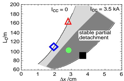
Fig. 2: Stable partial detachment is restricted to large  $\Delta x$  and small  $L_c$  ranges (shaded region). Four configurations are selected for numeric studies.
