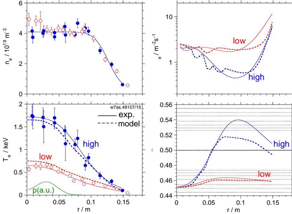
Fig. 3: Radial profiles for low and high confinement. Dashed lines: model. Full lines and data points: experiment (discharges with  $I_{p,0} = 0$  and 7.3 kA of Fig. 2 at  $t = 1.0$  s, data: Thomson scattering,  $e_e$  from power balance,  $-$ : calculated from bootstrap current normalized to plasma current). The assumed power density profile is indicated. Horizontal lines: rational  $-$ values up to  $m = 20$
