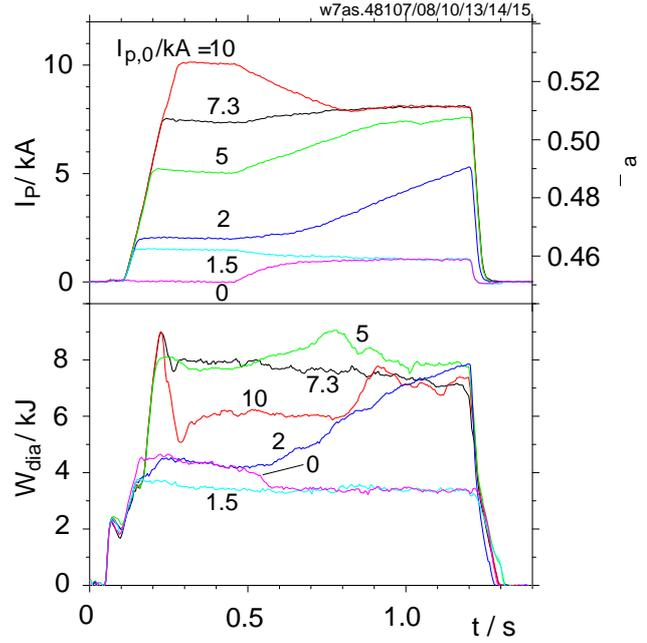
Fig. 2: Evolution of plasma current and diamagnetic energy for discharges with different initial inductively controlled currents. The external loop voltage is switched off at 0.45 s. ( $B = 2.5$  T,  $P = 400$  kW,  $n_e = 4 \times 10^{19} \text{ m}^{-3}$ ,  $-_{ex,a} = 0.45$ )
