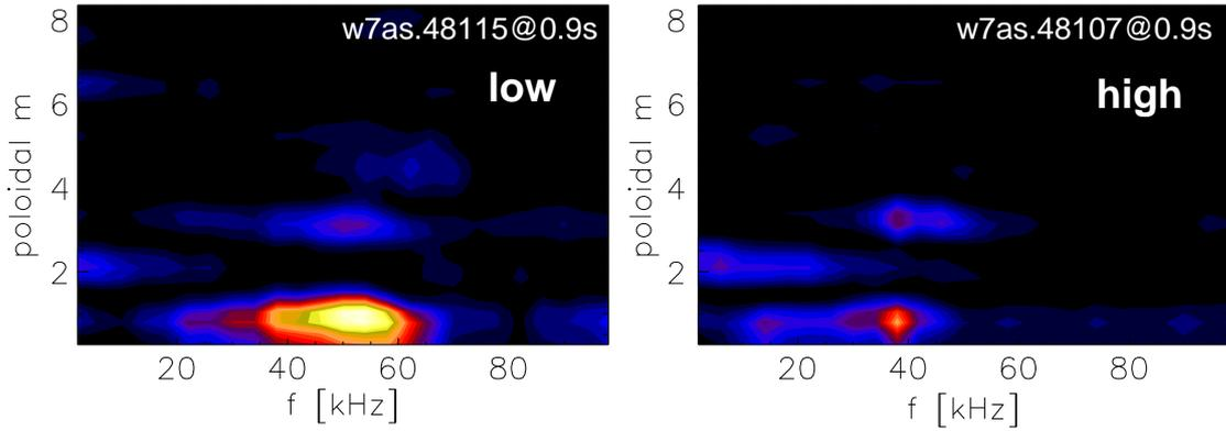
Fig. 4: Contour plot of magnetic fluctuation intensity measured by a poloidal array of 16 Mirnov probes as a function of frequency and poloidal mode number at low (left) and high (right) confinement.
