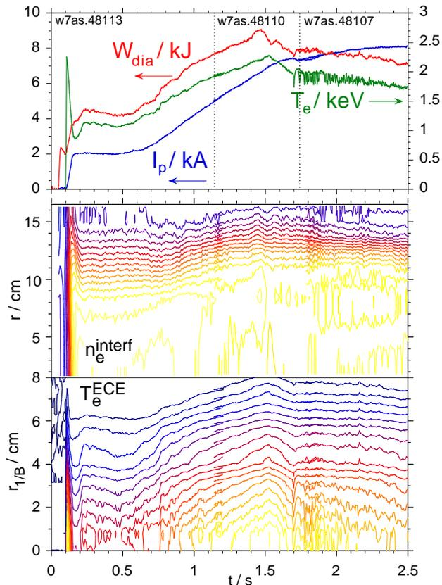
Fig. 5: Evolution to steady state plasma current at high confinement of  $W_{dia}$ ,  $I_p$  and central  $T_e$  (from ECE) and of the radial profiles of  $T_e$  and  $n_e$  (contour lines from interferometry and ECE,  $r_{1/B}$  is approximately  $0.5 r$ ). The extended timescale is obtained by shifting the traces of the  $2, 5$  and  $7.3$  kA discharges in Fig. 2 such that they continuously match.
