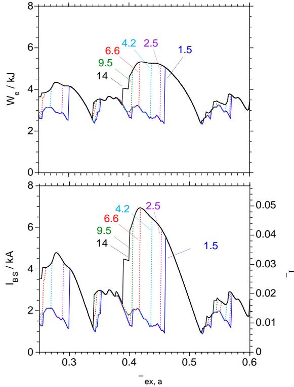
Fig. 1: Calculated dependence of electron kinetic energy and bootstrap current on  $-_{ex,a}$  showing two branches of confinement. The curves are labeled by the bootstrap current corresponding to the initial  $T_e$ -profile for the iteration. ( $B = 2.5$  T,  $P = 400$  kW,  $n_e = 4 \times 10^{19} \text{ m}^{-3}$ ,  $I_{OH} = 0$ ,  $r_{dep} = 0$  cm)
