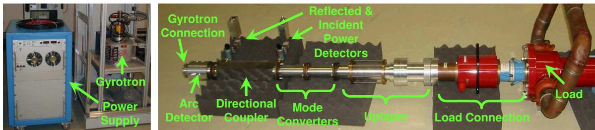
Figure 7: Left: CPI Gyrotron with IPF Stuttgart power supply. Right: Transmission line assembly for the gyrotron load tests. Load and adaptor components kindly loaned by CIEMAT Madrid. New components designed by IPF Stuttgart and manufactured at IPP Greifswald.
