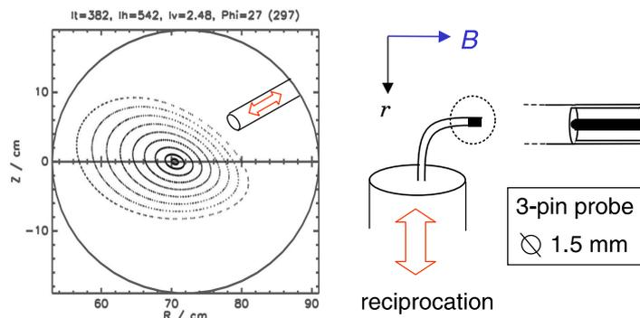
Figure 3: Schematic of the probe measurement system. On the left a cross section of WEGA's magnetic surfaces at  $\iota/2\pi \approx 0.2$  is shown, together with the radial movement of the probe system. On the right the 3-pin probe is shown in a vertical view. The 3-pin probe consists of a central detection pin and two flank-
