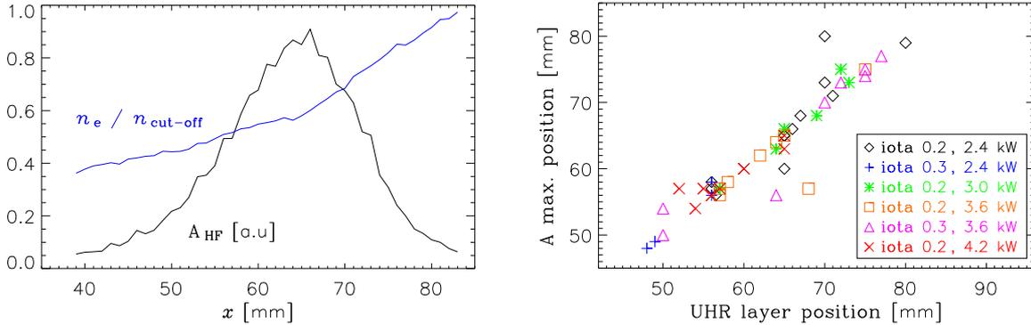
Figure 4: Results of probe measurements in WEGA. On the left: Amplitude of the 3-pin probe signal as a function of probe position. Overplotted is the plasma electron density, normalised to the O-mode cut-off. On the right: Correlation plot of the location of the maximum in the 3-pin probe signal, and the location of the UHR. Different colours correspond to different magnetic configurations and different heating power.
