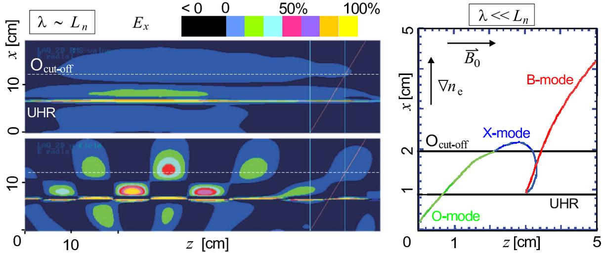
Figure 2: Comparison of the full wave calculation of the O-SX mode conversion with OXB ray tracing [4]. Different scale lengths are used. Left: Upper half is the time average of the  $x$  component of the electric field intensity  $E_x$ . The lower half is a snapshot of the  $E_x$  amplitude, displaying positive values only. Right: The ray trace path of the obliquely launched wave.
