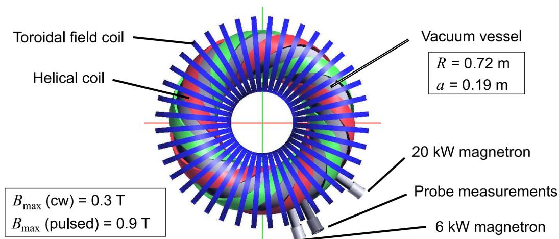
Figure 1: Top view of the WEGA machine, displaying the toroidal vacuum vessel (grey), and two coil systems. Also indicated are the ports for launching the microwave heating power and for doing probe measurements.
