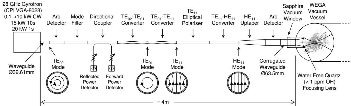
Figure 5: Schematic layout of the 28 GHz ECRH plasma heating system for WEGA. Layout and design of new waveguide components by IPF Stuttgart. Vacuum window and waveguide components kindly loaned by CIEMAT Madrid. New waveguide components manufactured at IPP Greifswald.
