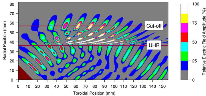
Figure 6: Time snapshot of the full wave calculation of the O-SX mode conversion for oblique launch of 28 GHz radiation into the WEGA plasma. Density increases linearly with radial position, magnetic field is parallel to the toroidal axis and, for clarity, only the positive electric field wave amplitude is shown.
