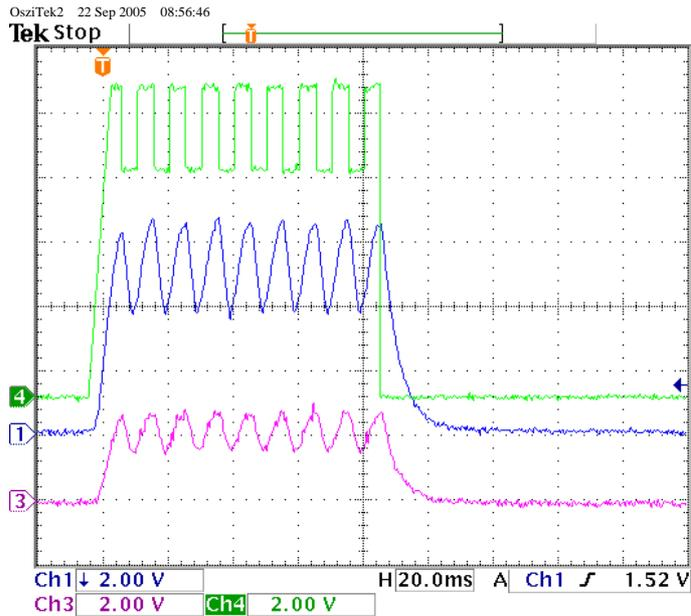
Figure 8: Gyrotron power supply full power modulation test results. Shown are the input voltage control signal, Ch4, and the measured output voltage, Ch1, and current, Ch3, across a large  $2.77 \Omega$  resistor. For Ch1, each division corresponds to 10 kV, while for Ch3 each division corresponds to 0.72 A. The 24 to 34 kV output voltage from the power supply corresponds to 0.1 to 20 kW power output from the Gyrotron.
