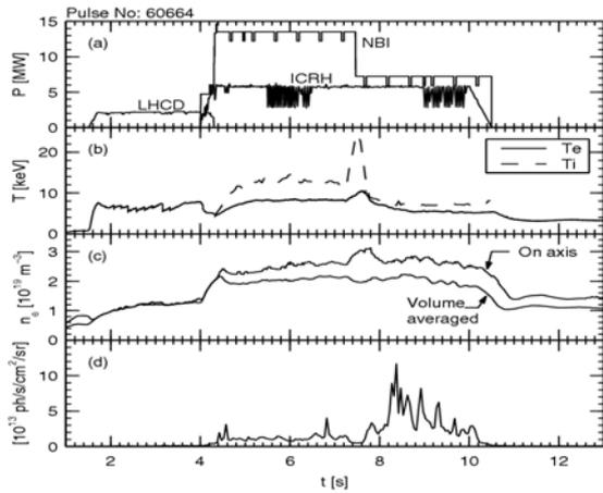
Fig. 1. Time traces for #60664. (a) NBI, ICRF and LHCD power, (b) central electron,  $T_e$ , ion  $T_i$ , temperature, (c) on axis and volume averaged electron density,  $n_e$ , and (d) BeII line radiation intensity.
