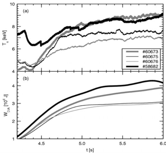
Fig. 2. a) Central electron temperatures and b) diamagnetic energy, for #58682 with 4.4MW +90° 51MHz, #60673 with 3.1MW dipole, #60675 with 5.2MW +90° and 60676 with 5.3MW -90°.
