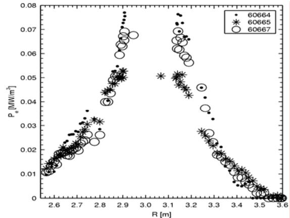
Fig. 3. Power deposition by direct electron heating obtained with modulation between 5.5 and 6.5s for #60664 with 5.3MW -90°, #60665 with 4.8MW +90° and #60667 with 2.9MW dipole.
