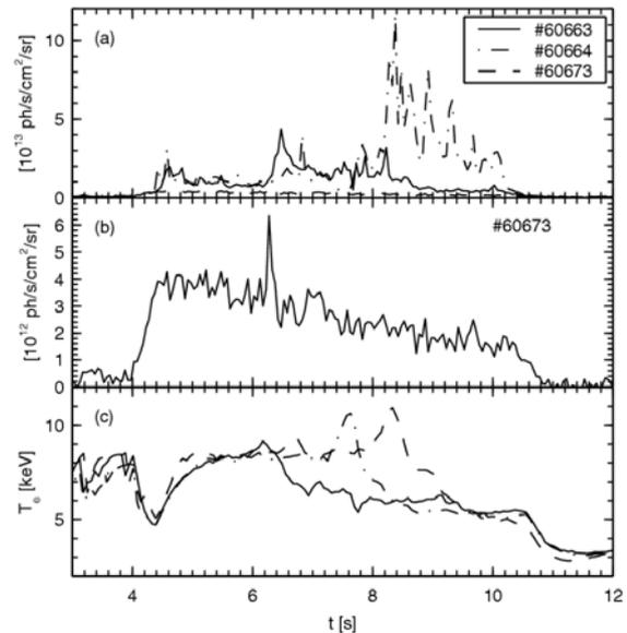
Fig. 4 a) and b) BeII line radiation intensity for a sight line passing through the inner divertor c) central electron temperature for #60663 (+90°), #60664 (-90°) and #60673 (dipole).
